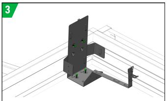
Select the right type of screw ( $\emptyset$  8-6 mm) depending on the base material. Attach the holder to the base with two screws and at least two to the side (the screws are not included). If it is not possible to attach to opposite side, four screws should be used to the side where this is possible
