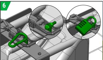
To prevent the holder from opening accidentally, for additional safety, hook a carabiner into the clamp loop, screw in the M6 screw with a nut, or lock it with a padlock (not included in the kit)
