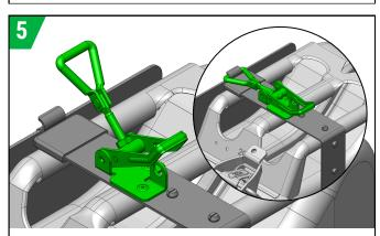
Hook the connection latch and then press the lever. If the lever cannot be locked or left free movement after pressing, adjust the length of the mechanism loop by screwing or unscrewing it from the hinge. It is not recommended to leave the holder under precipitation for a prolonged period
