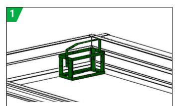
Select a safe position for the cans holder where it will be attached. When installing on a vehicle, please observe the legal requirements for add-on parts. If in doubt, contact the relevant authority for clarification
