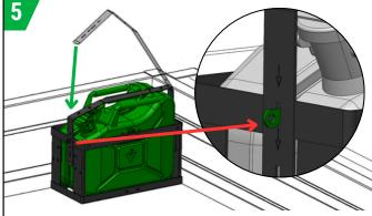
Hook the latch over the clamp loop and ensure it is fully secured. It is not recommended to leave the holder under precipitation for a prolonged period
