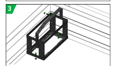
Select the right type of screw ( $\emptyset$  8-6 mm) depending on the base material. Attach the holder to the base with two screws and at least one to the side (screws not included). Attaching a holder only from the side is not allowed
