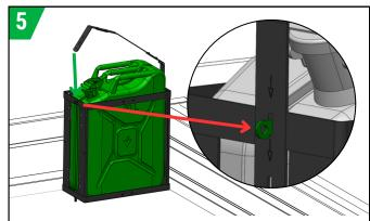
Hook the latch over the clamp loop and ensure it is fully secured. It is not recommended to leave the holder under precipitation for a prolonged period
