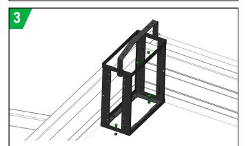
Select the right type of screw (Ø 8-6 mm) depending on the base material. Attach the holder to the base with two screws and at least one to the side (screws not included). Attaching a holder only from the side is not allowed
