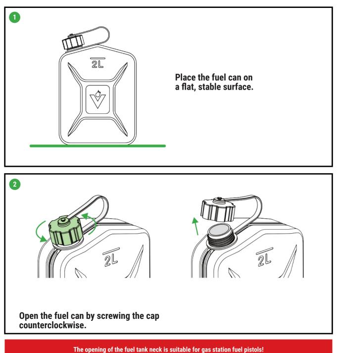
CAUTION! Fill slowly. If the fuel tank is filled quickly, fuel spillage is possible.
